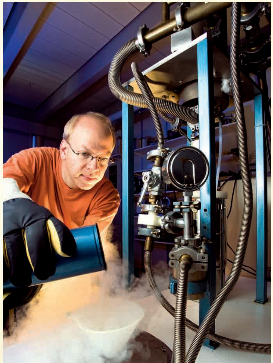
Filling a cryostat with liquid air. In this apparatus silicon-carbide transistors for high-power electronics are examined.
