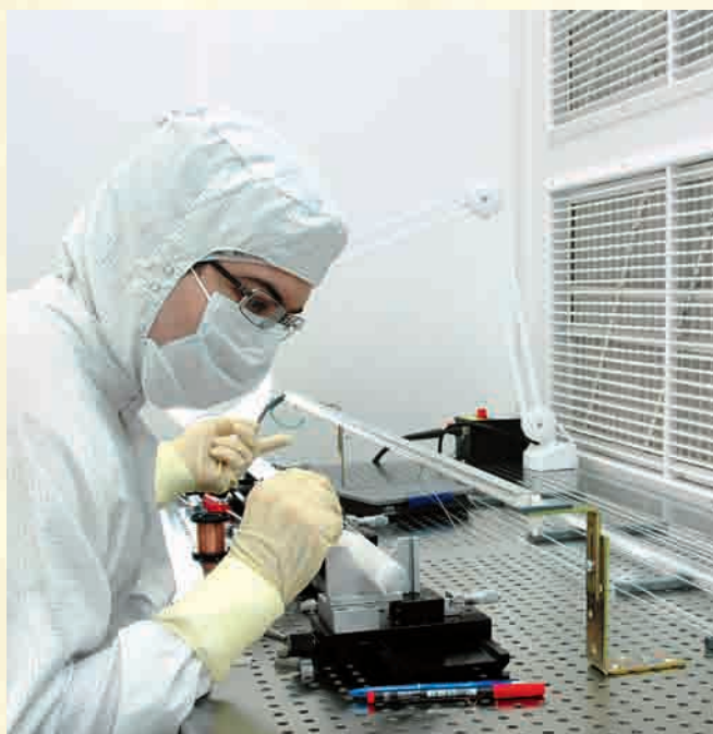
Fabrication of photonic crystal fibers.
