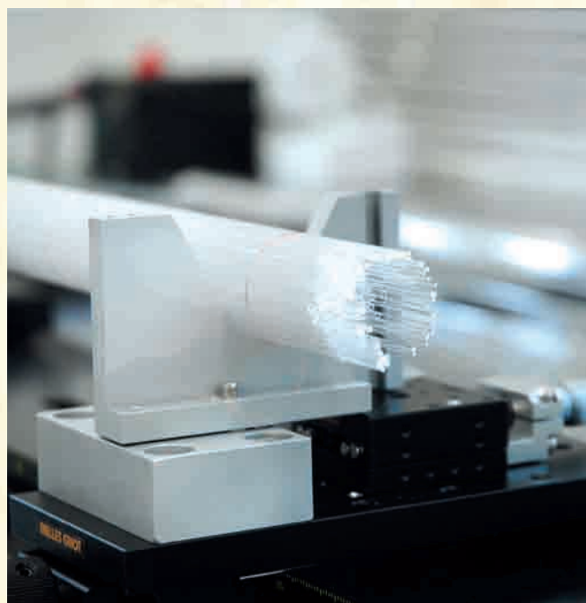
A stack of glass rods and tubes as preform for drawing fibers.
